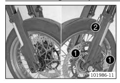
Position the fork protection on the left fork leg. Mount and tighten screws ①. Guideline
