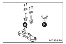
In the upper triple clamp, there are 2 drill holes separated by a distance of  $oldsymbol{A}$ .
