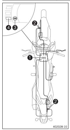
The ABS unit 1, which consists of a hydraulic unit, ABS control unit, and return pump, is installed under the seat. A wheel speed sensor 2 is located at the front and rear wheels.
