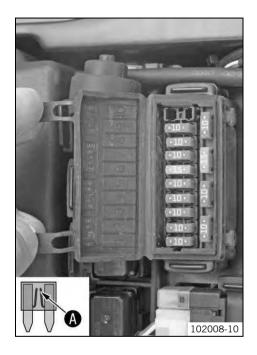
Remove the defective fuse
