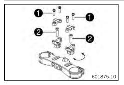
Remove the four screws ①. Remove the handlebar clamps. Take off the handlebar and set it aside.
