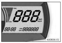
When you switch on the ignition, all display segments light up for a second as a function test.
