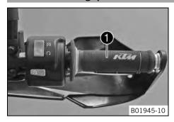
The throttle grip **1** is fitted on the right side of the handlebar.
