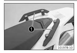
The handrails **1** are used for moving the motorcycle around. When you have a passenger, the passenger can hold on the handrails during the journey.
