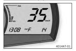
If the fuel level drops to the reserve mark, the display automatically changes to  $TRIP\ F$  and starts to count from 0.0, regardless of the previous display mode.
