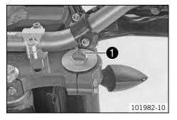
Turn the red adjusting screw 1 all the way clockwise.
