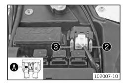
Remove a defective main fuse 2 with needle nose pliers.
