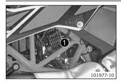
The seat can be released using strap **1**.
