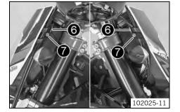
Position brake line guides **6**. Mount and tighten screws **7**. Guideline
