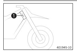
The chassis number 1 is stamped on the steering head on the right.
