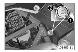
Turn adjusting screw 1 clockwise all the way using a socket wrench.
