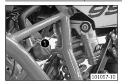
The shock absorber part number **1** is stamped on the top of the shock absorber above the adjusting ring on the engine side.
