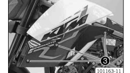
Position the spoilers on both sides. Mount and tighten screws 3.
